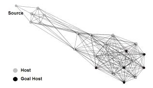
Figure 4: Connectivity graph of a network. Each node is a host computer, a directed edge between two hosts (u, v) means host u can initiate a connection to node v
