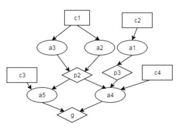
Figure 1: Example of an attack graph
